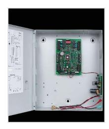
The VRC-2000 Intelligent Field Panel utilizes flash firmware for easy upgrades, and employs fully distributed intelligence for off-line operations. The panel contains on-board clock and memory backup as well as thermal overload protection.
